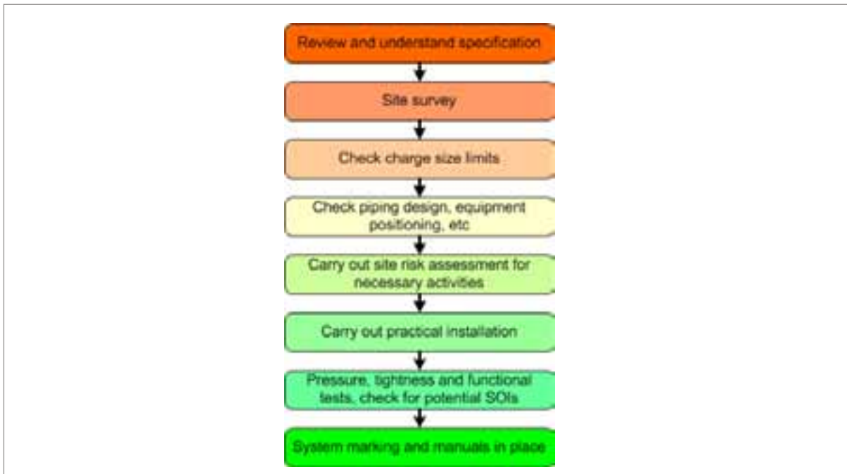
Figure 68: General procedure for installation of systems and equipment
