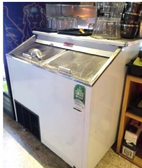
Photo 12: Example of Industrial ice storage with R-290, © GIZ/Philipp Denzinger.
