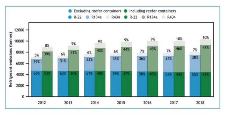
**Figure 60** – Estimated refrigerant emissions of the global fleet, showing both totals when including and excluding reefer containers
