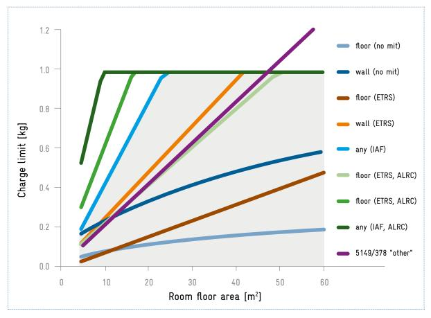
Figure 2: Example of the relationship between room size and refrigerant charge limits using different risk mitigation methods. For example, with integrated airflow (IAF), any charge for the room size within the shaded area is permissible.
